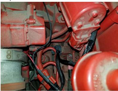
**8)** Plug the Ag Diesel Solutions female MAP sensor connector into the stock male MAP sensor. Plug the Ag Diesel Solutions male MAP sensor connector into the stock female MAP sensor connector.
