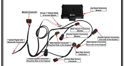
1) At the rear of the RV, locate the 3 sets of stock injector connectors attached to the side of the engine head. These are located on the same side of the engine as the air intake. One connector is located closer to the Flywheel-side of the engine, one is in the middle behind the air intake, and the last connector is located closer to the Fan-side of the engine.
