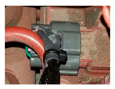
9) Connect the red wire with ring terminal to a +12V constant source, such as the intake air heater grid relay. Connect the black
