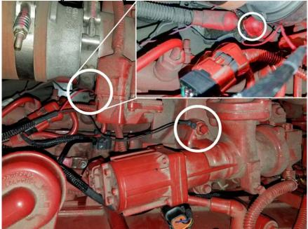
**10)** Plug the Harness into the module. Mount the module with supplied zip ties away from any excessive heat or moving parts. Note: Zip tie the module to the factory wire harness. Mounting the module with the switch connector down will help prevent moisture from collecting into the module connector.
