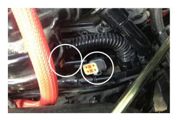
**3)** Route the Module Harness as shown in the picture below. The Module Case will be located closer to the Flywheel side of the engine.
